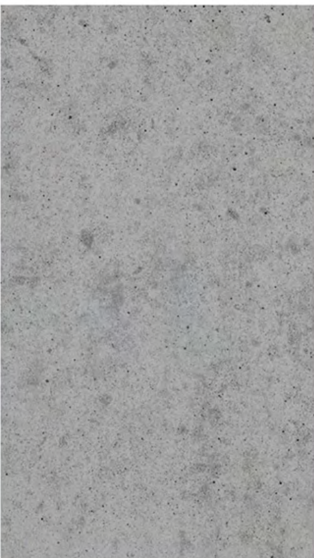
Smooth Poured in Place Concrete
